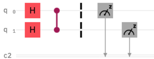
Figure 1.2: Quantum circuit representing uniform probability distribution with entangled qubits.
